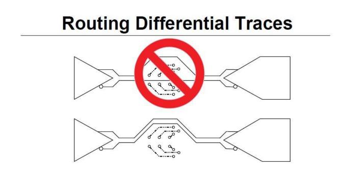
It is also good practice to keep adjacent differential signal traces close together, and away from traces carrying power to minimize interferences. Another tip is to avoid 90° angles in traces and instead to use chamfers or  $45^{\circ}$  angles whenever the traces must change direction.
